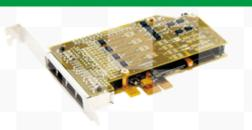
Synway open source family includes four product lines: FXM series analog telephony boards, TEJ series digital telephony boards, CDC series boards for transcoding, chassis-based Asterisk appliance. The open-source family reassures high interoperability, voice quality and robustness. All these Asterisk hardware platforms adopt Synway's patent-pending echo cancellation technology SuPerForm(128ms echo tail).
