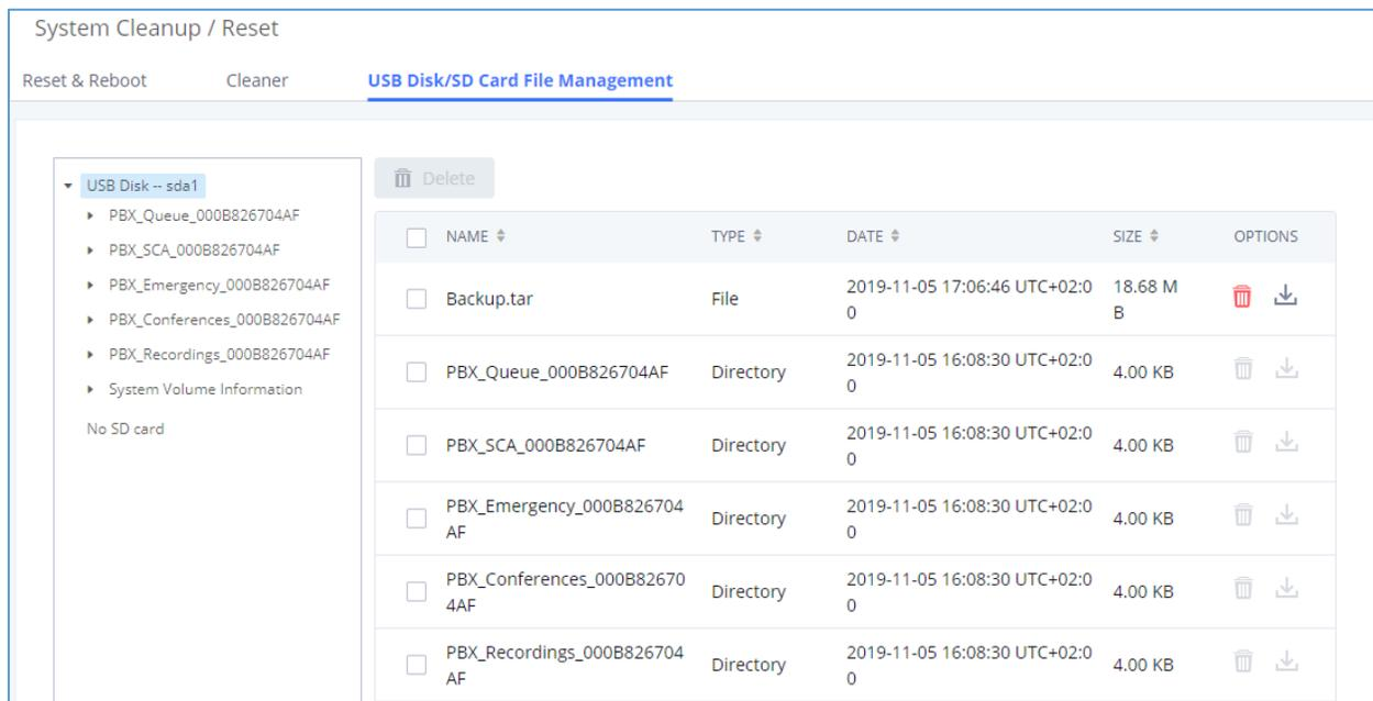
The screenshot shows the 'System Cleanup / Reset' page with the 'USB Disk/SD Card File Management' tab selected. On the left, a tree view shows the contents of 'USB Disk -- sda1', including directories for PBX\_Queue, PBX\_SCA, PBX\_Emergency, PBX\_Conferences, and PBX\_Recordings. A 'Delete' button is visible above the file table. The table lists files with their names, types, dates, sizes, and options to delete or download.
