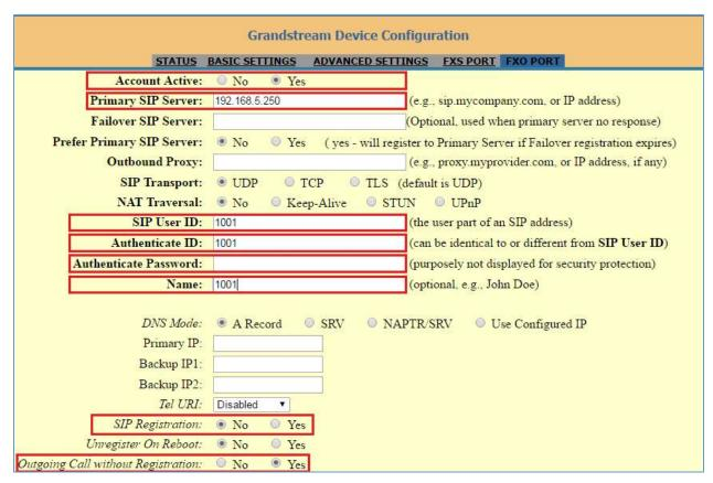
Figure 14: Configure FXO Port on the HT503 - Registration
