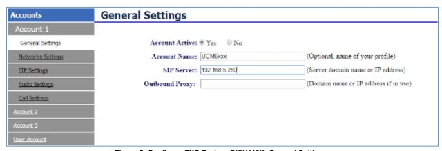
Figure 5: Configure FXO Port on GXW410X: General Settings
