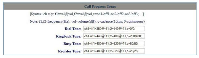
Figure 10: Configure FXO Port on the GXW410X: Call Progress Tones
