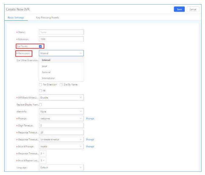
Figure 5: Create an IVR on UCM6XXX - Dial Trunk Enabled
