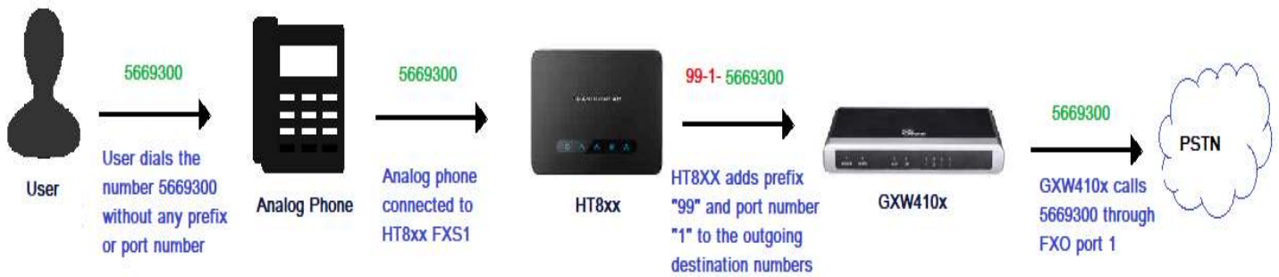
Figure 15: Port-To-Port Mapping call flow
