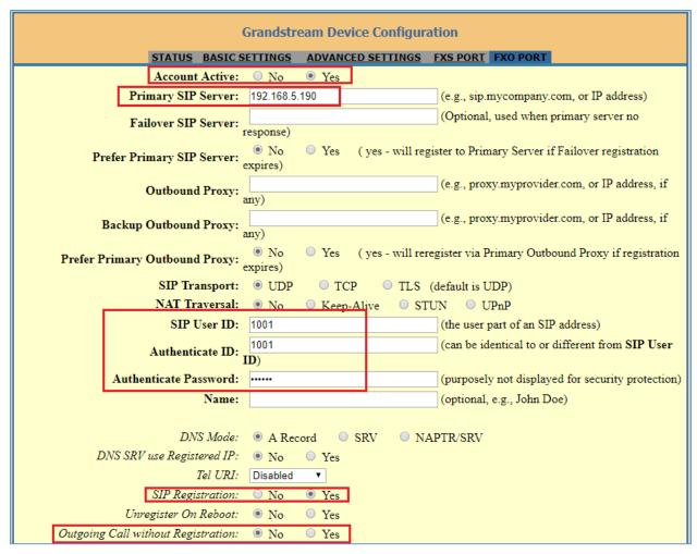
Figure 6: Configure FXO Port on the HT813 - Registration
