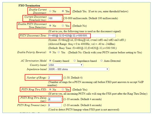
Figure 17: Configure FXO Port on the HT813: FXO Termination
