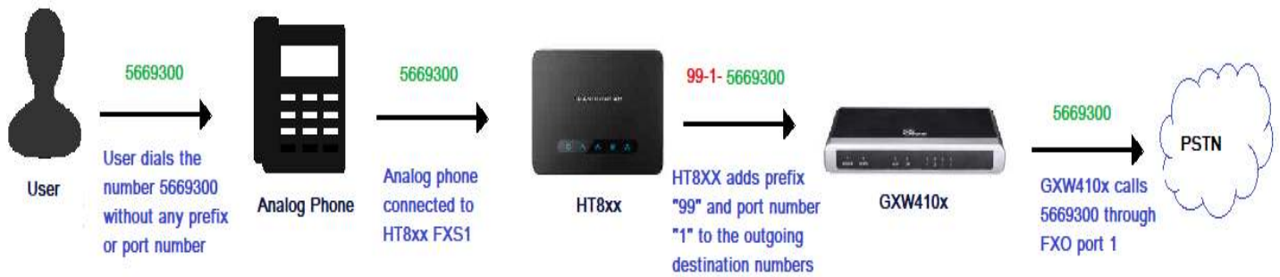
Figure 15: Port-To-Port Mapping call flow
