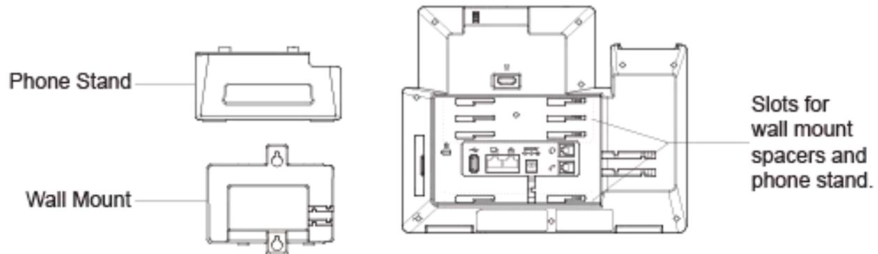
Figure 2: Phone Stand and Mounting Slots on GXV3350
