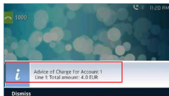
Figure 9: AoC-E displayed at the end of a call on GXP2135
