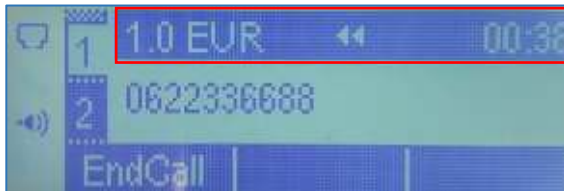
Figure 4: AoC-D displayed during a call on GXP1628
