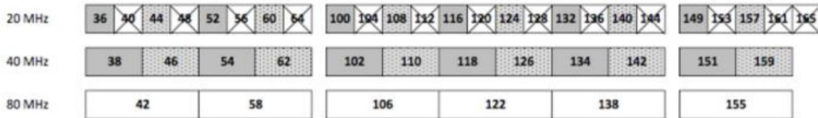
**Figure 18: Selection of 5G 20MHz primary channel**
