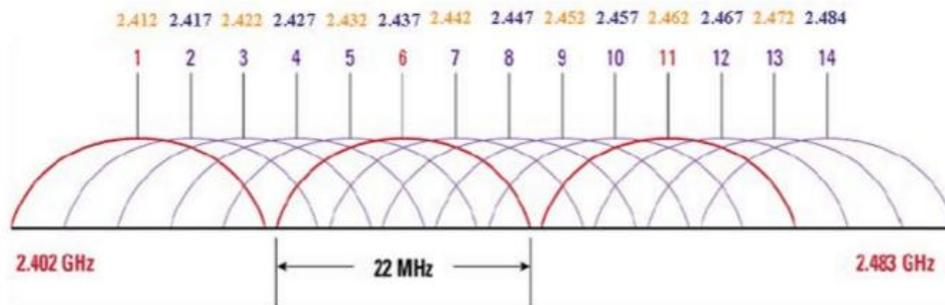
**Figure 5: Channels overlapping on the 2.4GHz**
