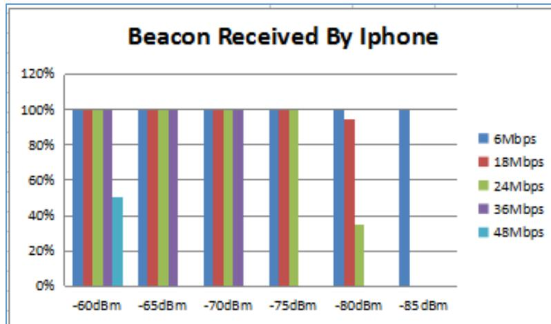
**Figure 9: Control cellular size of the AP by lowering the transmission power**
