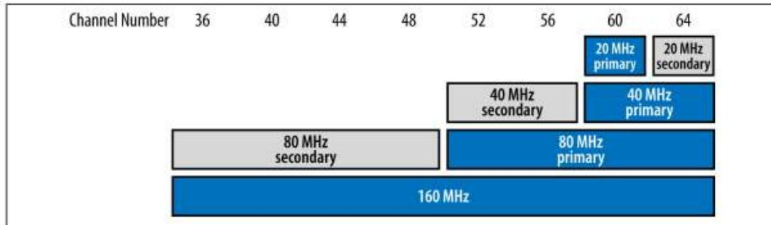
**Figure 17: 5G primary and secondary channels**
