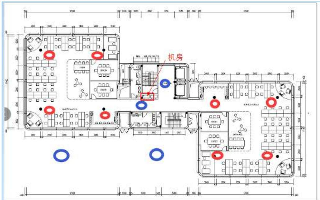
**Figure 1: Positions of Access Points deployed on the Floor Plan**
