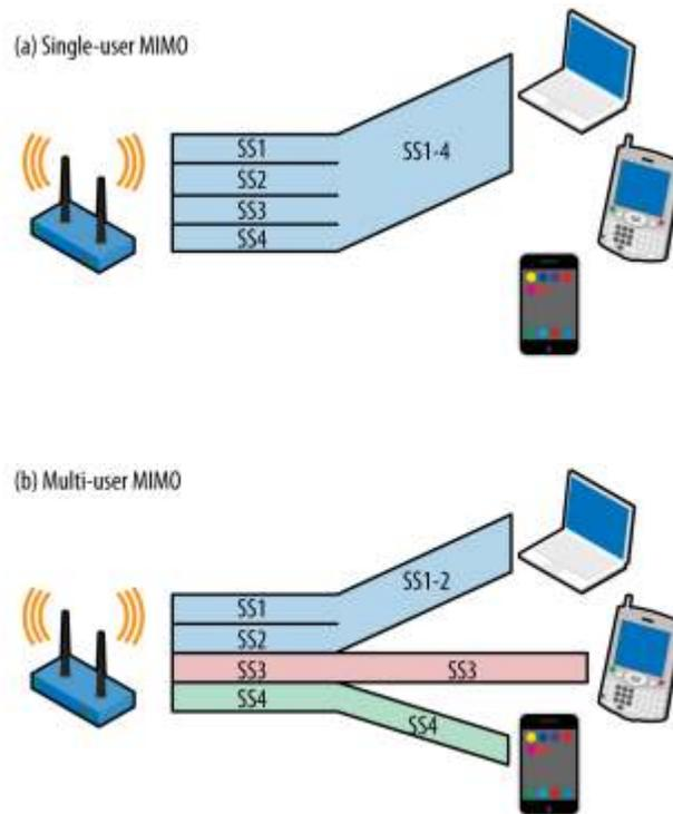
**Figure 12: Diagram of downlink transmission of SU-MIMO and MU-MIMO**
