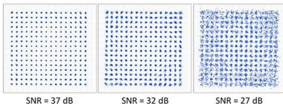
**Figure 10: Required SNR value in the 256QAM modulation mode**
