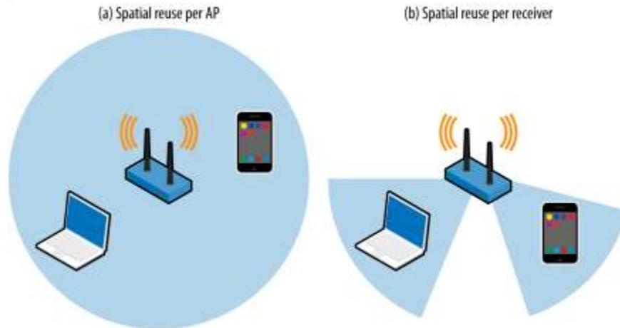
**Figure 13: SU-MIMO Omnidirectional antenna vs MU-MIMO beamforming**
