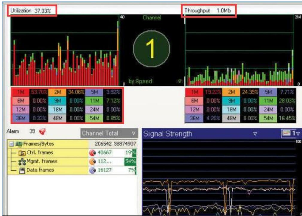
**Figure 8: External interference caused by other wireless appliances**
