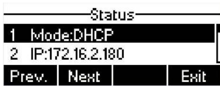
Figure 6 - Check the Device's IP Address
