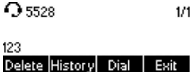
Figure 33 - Dial a Number after Audio Channel Opened
