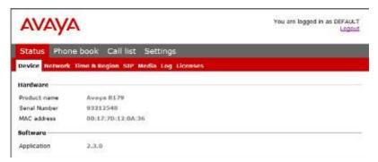
The Device tab shows phone information including serial number, network port and current software version.
