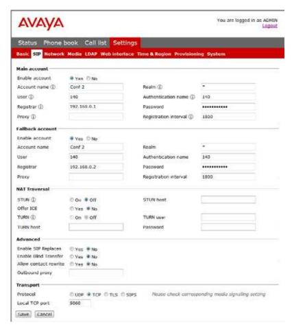
The conference phone supports two accounts. The second account is a fallback account that is automatically used if the phone fail to register to the main account. Note that this account then will be used as long as the fallback account is available. If the phone fails to register to the fallback account, it will try to use the main account again.
