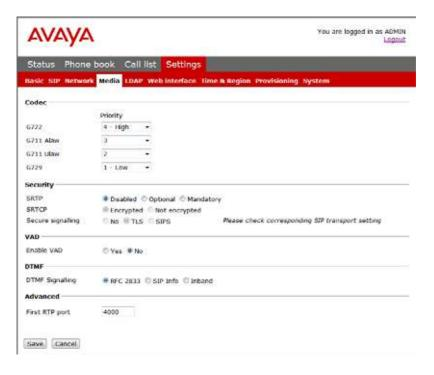
The media settings determine how audio is sent between the devices. The devices negotiate via SIP before a call is connected. All devices must support the same media types, codecs and security settings.
