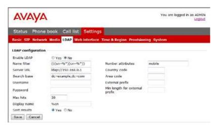
Avaya B179 has support for an external phone book, which means it can communicate with a directory server using LDAP (*Lightweight Directory Access Protocol*). The built in search function dynamically filters the content from the LDAP database, based on the search characters the user enter.
