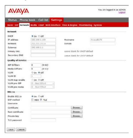
DHCP Dynamic Host Configuration Protocol is used by network devices (clients) to obtain the parameters necessary for operation in the IP network. This protocol reduces system administration workload, allowing devices to be added to the network with little or no manual configuration.
