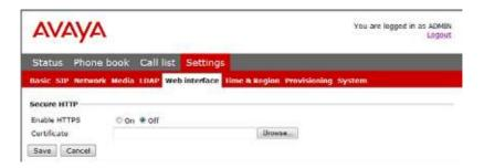
The web server in the Avaya B179 supports secure connections using HTTPS.
