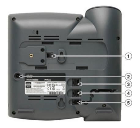
**Caution** Do not insert a telephone line cord into the port marked 'AUX' (1).
