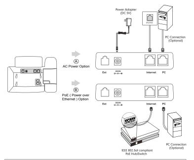
Note: If inline power (PoE) is provided, you do not need to connect the power adapter. Make sure the Ethernet cable and hub/switch are PoE compliant.
