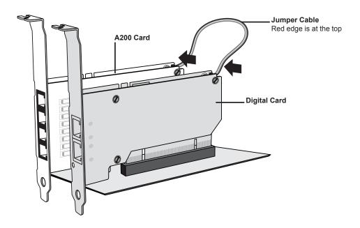
The digital card must have a HWEC (hardware echo canceller). The minimum firmware that supports clock synchronization for the A200 is v10. For more information, please go to <a href="wiki.sangoma.com/t1e1analogfaxing">wiki.sangoma.com/t1e1analogfaxing</a>
