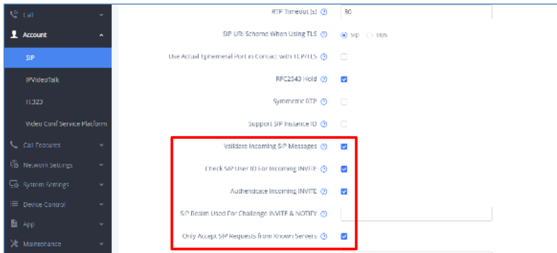
Figure 12: Settings to Block Unwanted Calls on GVC3220
