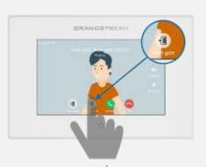
Video Intercom after doorbell pressed, GSC3570 virtual open door icon pressed to open door from inside
