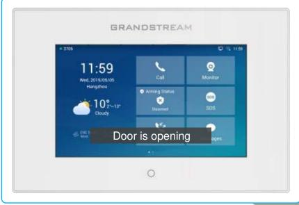
DI Zone type set to Open Door in Zone settings, wired to open door switch.
