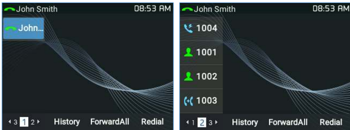
Figure 51: VPK - LCD Indication
