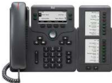
Figure 6. Cisco IP Phone 6800 Key Expansion Module
