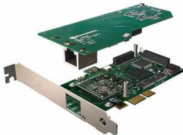
A101DE 1-port T1/E1/J1 shown with available echo canceller and PCI-Express interface
