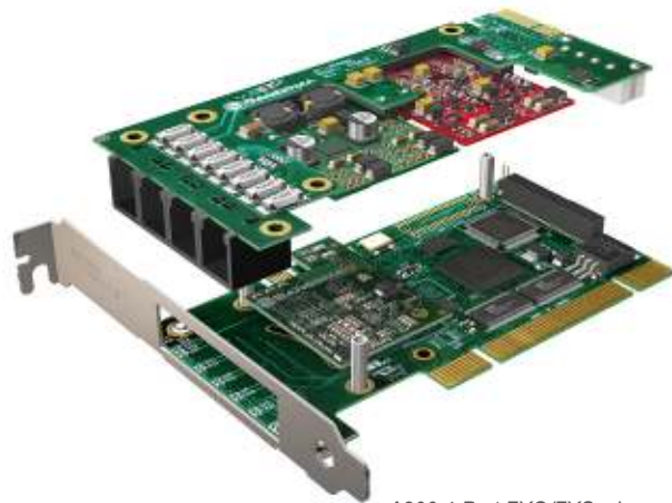
A200 4-Port FXO/FXS, shown with hardware echo canceller, disassembled
